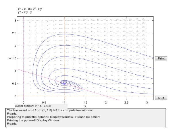
Figure 5.3.2: Sketch of Phase Portrait for System (5.71) with  $r=\beta=\gamma=1$  and L=2
