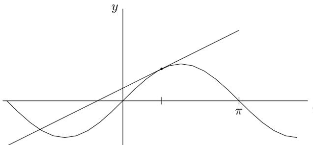
Figure 6.3.2: Sketch of graphs of  $y = \sin x$  and its tangent line at  $\left(\frac{\pi}{3}, \frac{\sqrt{3}}{2}\right)$
