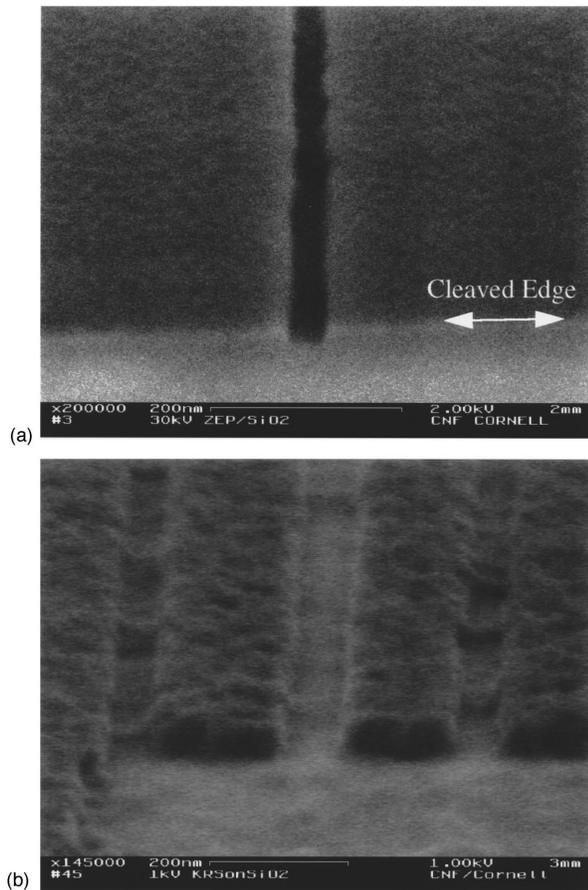
FIG. 4. Examples of the vertical sidewalls achieved using conventional RIE to transfer patterns from ZEP-520 (a) and KRS (b) into  $\text{SiO}_2$ . The ZEP-520 was exposed at 30 keV (line dose 30 pC/cm) and is shown in a cleaved cross section. The KRS pattern has single pass lines on each side of a finite-width line, and was exposed at 1 keV (line dose 18 pC/cm).
