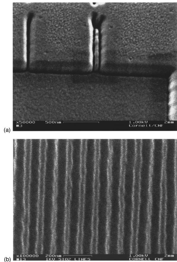
FIG. 5. Two examples of the narrow spacing possible using ZEP-520 on both Si (a) and  $\text{SiO}_2$  (b) substrates. The lines in Si are spaced 80 nm apart and were patterned at 2 keV (line dose 22 pC/cm). The grating in  $\text{SiO}_2$  has a 100 nm period and was exposed at 1 keV (line dose 15 pC/cm).
