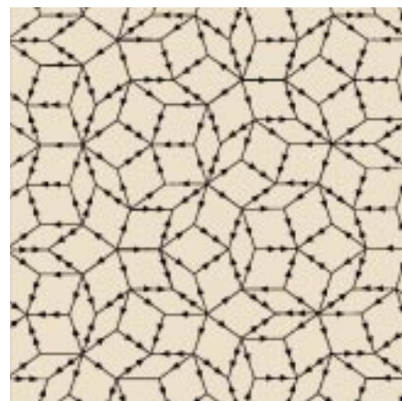
Figure 1 Penrose's planar quasiperiodic tiling. It is formed by a set of two rhombuses with edges of equal length, one with angles of 36° and 144° and one with angles of 72° and 108°. Their edges are marked with single or double arrows, and the rules constrain adjacent tiles to have matching arrow types along their shared edge.
